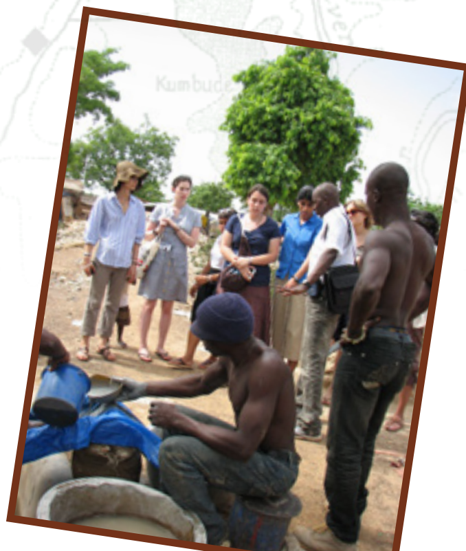
Undergraduate students from initial U-M 2009 trip, watching miners refine the stone-gold powder mixture before adding mercury, at the small-scale gold mining site called Kejetia, in the Talensi District
