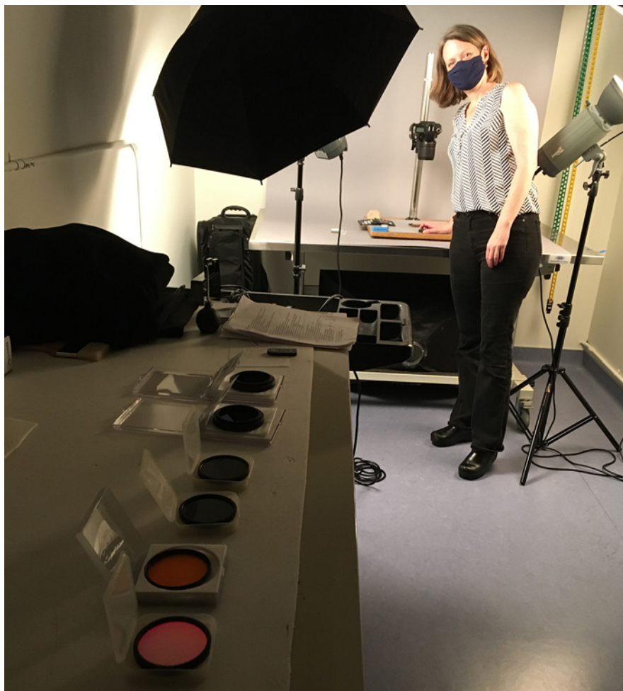
Figure 3. Conservator Suzanne Davis prepares to use multispectral imaging (MSI) to investigate dyes on an ancient textile; lens filters for use on the MSI camera are arrayed in order of use along the table in the left foreground. Photo by Carrie Roberts.
