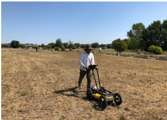
Figure 11. Dr. Nikos Papadopoulos of the Foundation for Research and Technology, Hellas, performs ground-penetrating radar survey at Pella (Greece) in July 2022. Photo by David Stone.
