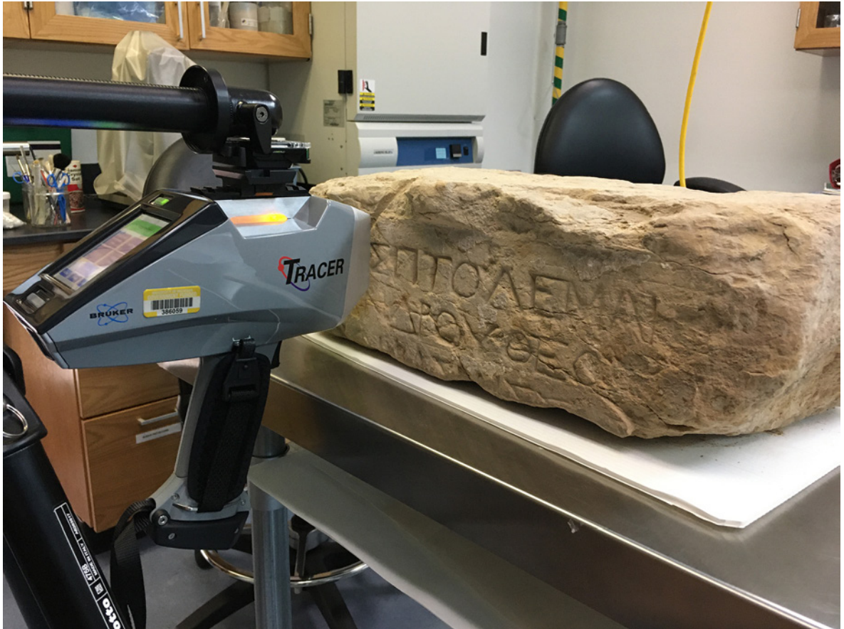
Figure 2. Portable X-ray fluorescence unit, set up and ready to study pigments and ground layers on an inscription from Karanis. Photo by Carrie Roberts.
