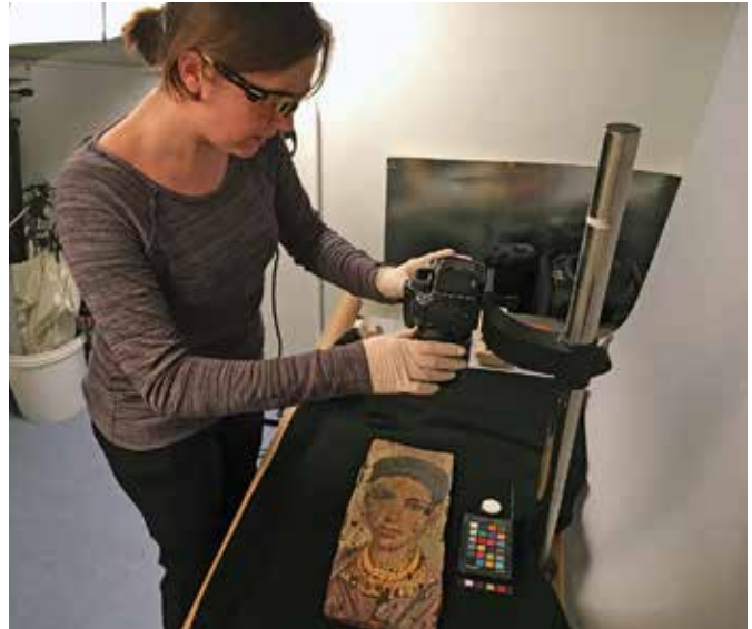
Carrie performing visible-induced infrared luminescence imaging on the Fayum portrait using a modified DSLR camera. Photo by Amaris Sturm.
