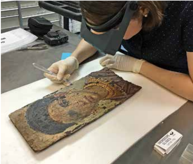
Carrie removes a miniscule paint sample from the Kelsey's Fayum portrait (KM 26801) for PLM and FTIR analysis. Photo by Amaris Sturm.
