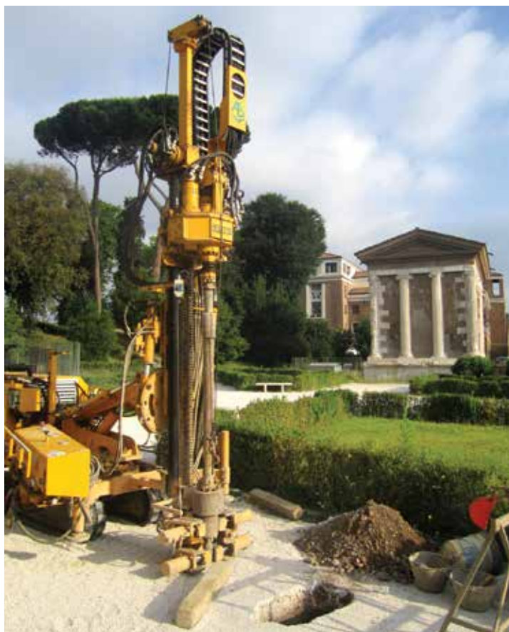
SOME OF THE EQUIPMENT USED TO DRILL CORE SAMPLES, WHICH HELP RESEARCHERS CONNECT THE DEVELOPMENT OF ROME TO THE ENVIRONMENTAL HISTORY OF THE AREA AROUND THE CITY.
